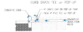
This modification to the downspout leader, along with regular maintenance, will enable water to get to the road and not back up along the foundation.
